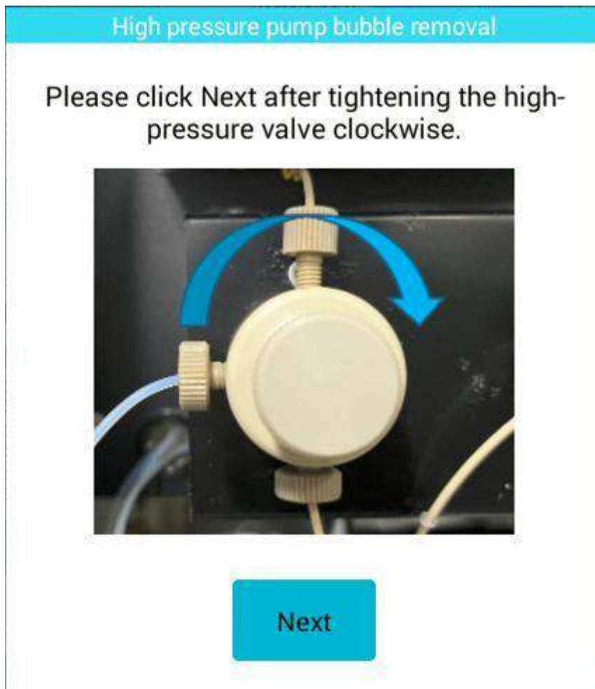
Figure 3-11 Tighten the high pressure valve clockwise
