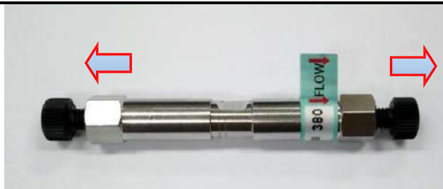
Figure 9-4 Remove the plus of new chromatography column
